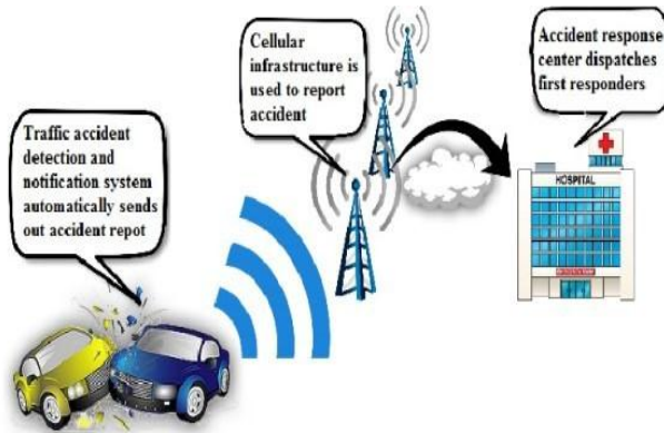
Fig 1. Traditional accident detection system using a smartphone
