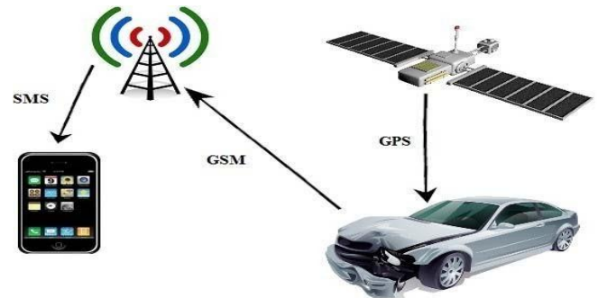
Fig 3. Accident Detection scheme through GSM and GPS
