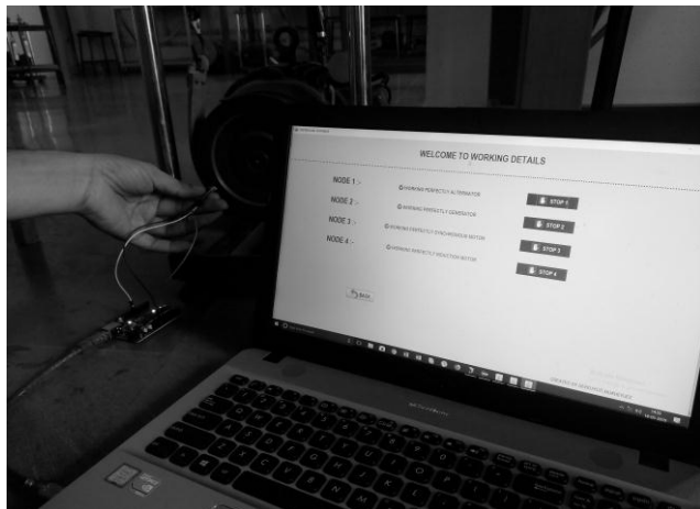
Figure 2. Hardware interfacing system with Arduino UNO
