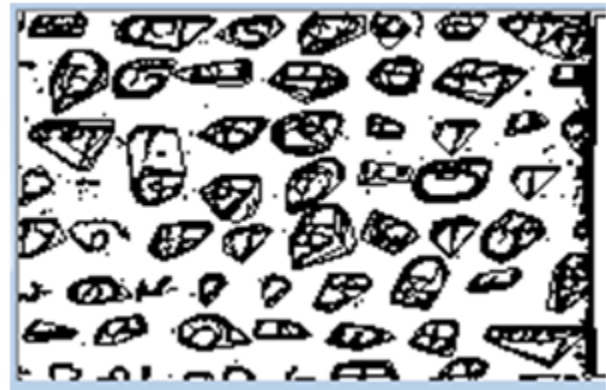
Figure4. Points marked to detect the characters using contour based convex hull bounding box segmentation.
