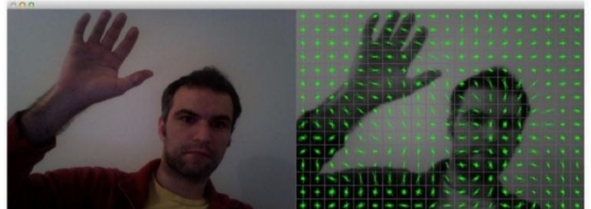
Fig.7: Example of an image for Gradient Histogram – each block contains 9-bin histogram for each 36 per block[6][7][25][28]
