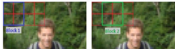
Fig. 6: Example of an image for Gradient Histogram for each block (4 cells with a 9-bin histogram)[25][28]
