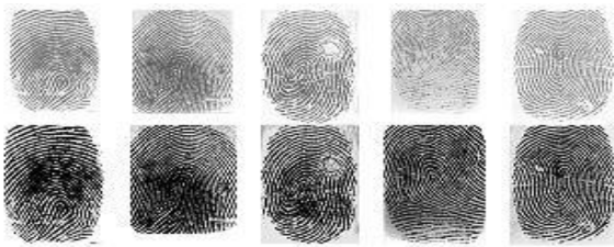
Figure 2. Original images are shown in row 1, whereas second row shows their corresponding normalized images.
