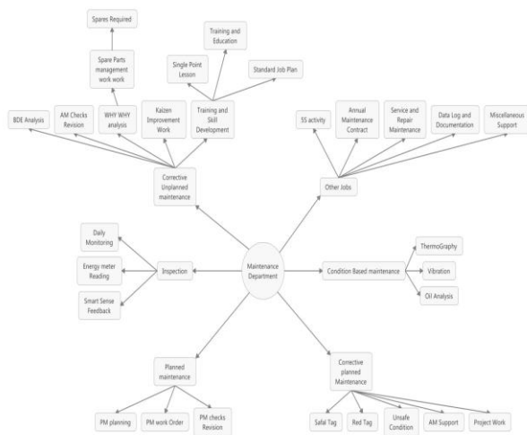
Figure 1 Structure based on CMMS Job type
