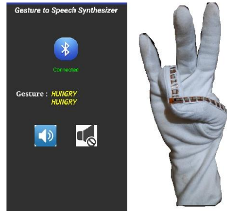
Fig 6 :android application screen shot and gesture for 'hungry' made through glove
