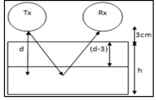
Figure 3. Finding the Garbage level using Trigger and echo signal HCSR04 Ultrasonics Sensor
