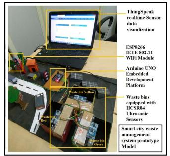
Figure 6. Implementation of Hardware prototype
