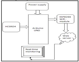
Figure 1. Block diagram of proposed Waste Management System
