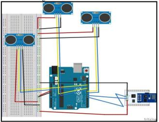
Figure 5. HCSR04 and ESP8266 ( IEEE 802.11 Wireless network Adpator) interfacing with Arduion UNO using Fritzing
