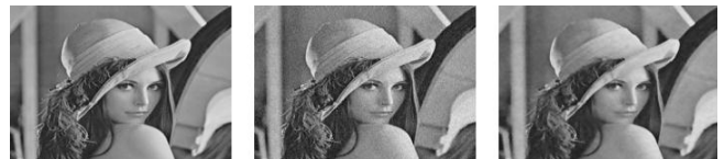
(a) Original Image (b) Noised Image Sigma= 30 (c) Denoised Image
