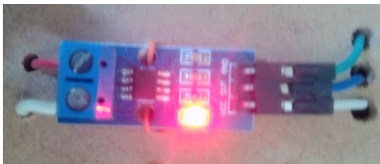
Figure 2. ACS712 Hall Effect Current Sensor
