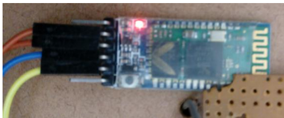
Figure 6. HC-05 Bluetooth Module.
