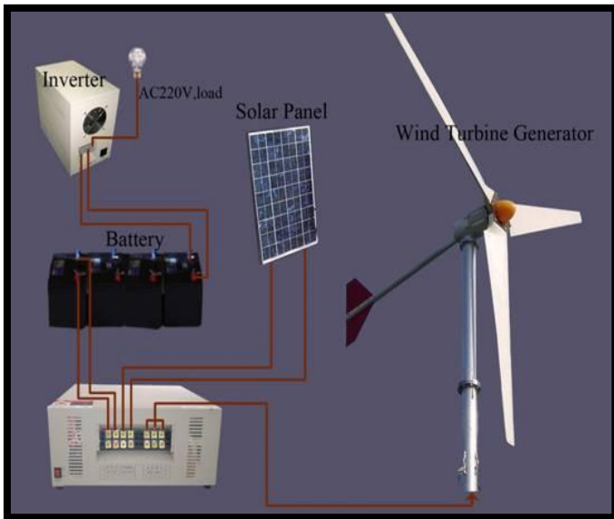
Figure 7-a Solar-Wind Hybrid System
