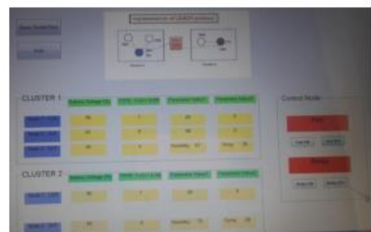
Fig 5- GUI of monitoring center showing the battery voltage and type of node as CH
