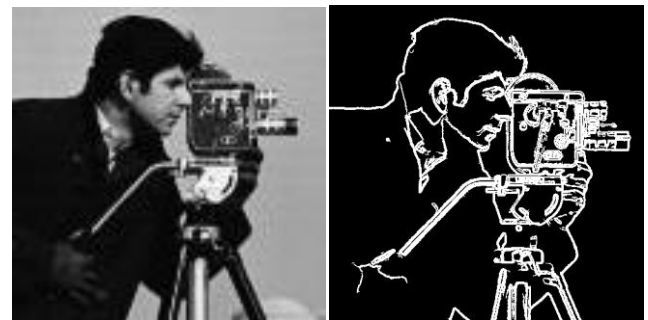
Figure 11. Sobel Edge Detection [10]
