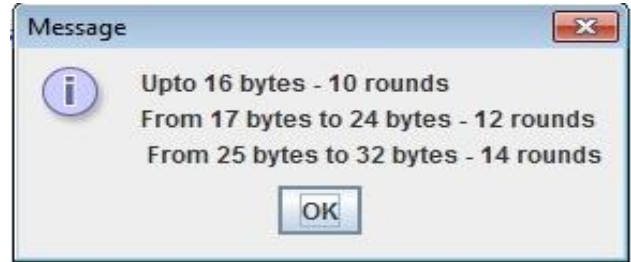
Fig15. displays the number of rounds the encryption/decryption process will undergo in each category
