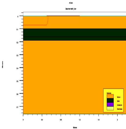
Figure-1 HBT structure for (base width = 90nm)
