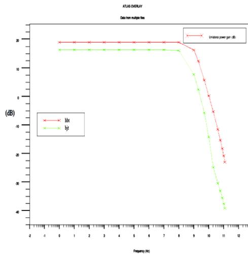
Figure-9 Comparison between HBT and BJT Power Gain Vs Maximum Oscillation Frequency
