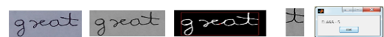
Figure 9. (a) Original Image; (b) Gray Image ;(c) Binary Image;(d) Segmented T-letter Image; (e) SVM Classified Output for Human Behavior
