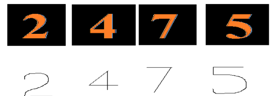
Figure 6: some examples of the thinning process using the Stentiford Algorithm
