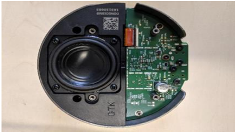
Figure 5. Loudspeaker and circuit board after removal of the covers
