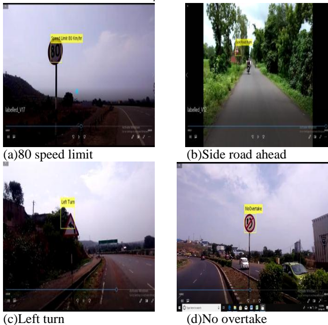
Figure 2. Screen shots of output video in avi format obtained by identification and recognition using ACF. (a) 80 speed limit, (b) Side road ahead, (c) Left Turn, and (d) No Overtake, are the few signage's obtained from experimentation.
