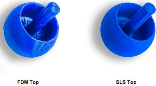
Figure 5: FDM vs SLS produced surfaces
