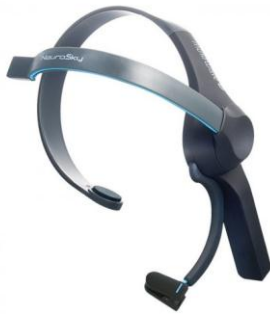
Figure 2. Neurosky MindWave Mobile EEG Headset
