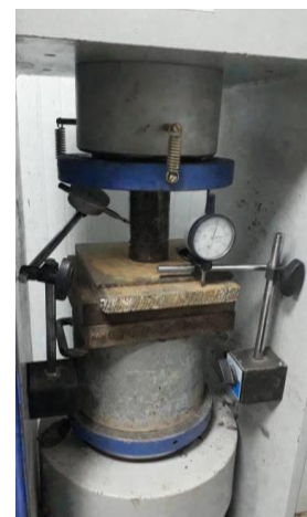
Photo. 5- Testing of Uniaxial Compressive Strength of ore sample (Omran Geotechnical Company. Kabul. 2017)
