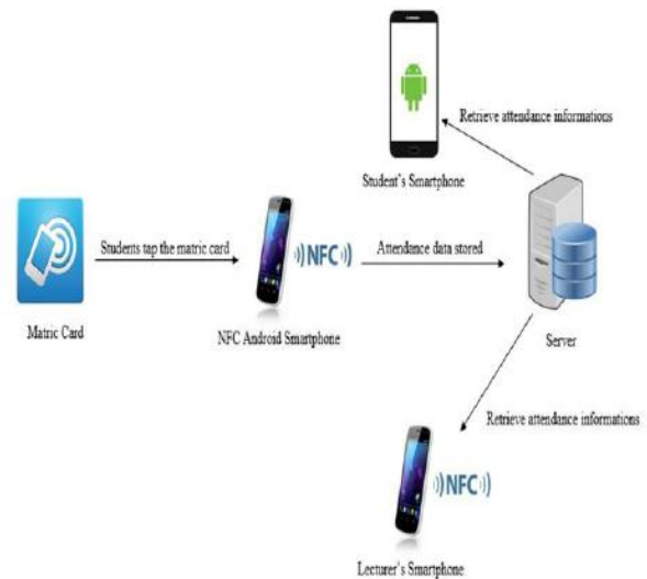
Fig: 1 Attendance system using NFC
