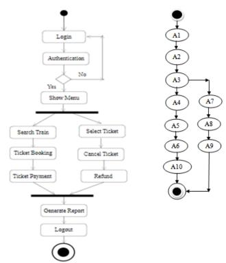
Figure 3(a) AD Railway Reservation system (b) ADG for Railway Reservation system
