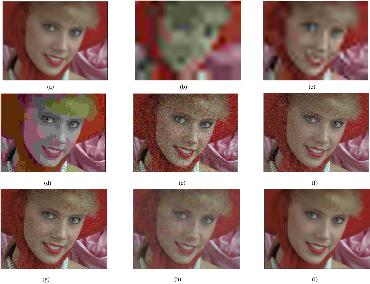
Fig. 7 Noisy test images from TID2008 database which are to be classified. Distortion types of (a) ~ (i) are “High blurring”, “JPEG 2000 compression”, “Quantization noise”, “JPEG compression”, “Spatially correlated noise”, “Impulse noise”, “additive Gaussian noise”, “image denoising”, and “Gaussian blur” respectively.
