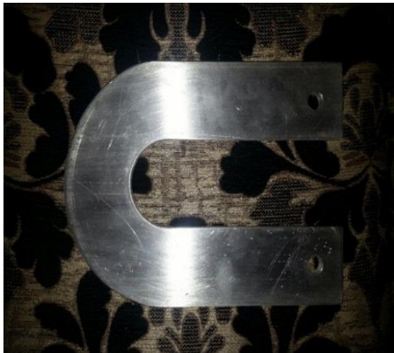
Fig. 4. Fabricated Curved Beam Specimen
