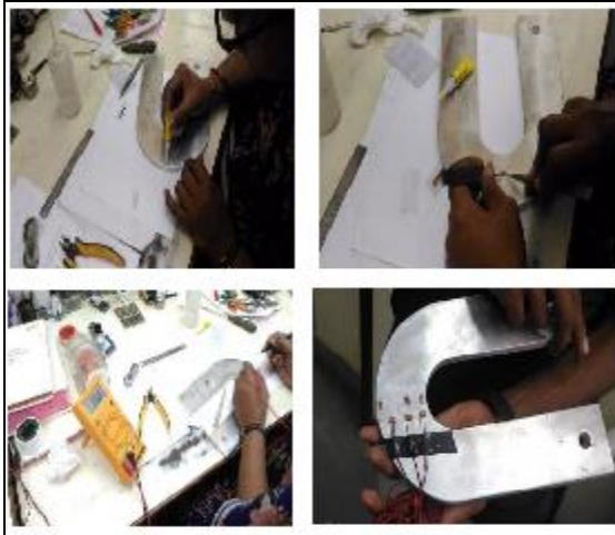
Fig.6. Strain Gauge Mounting Procedure
