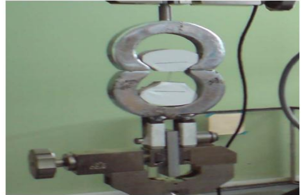
Fig. 3: briquette testing machine to determine the tensile strength of mortar.
