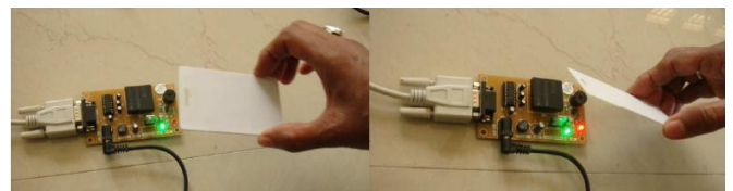
Figure 3. Detection of RFID tag by the RFID reader
