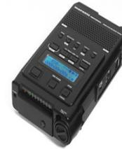
**2.2.10: Marantz PMD 660:** Recording Format: WAV, MP3, Memory: CF Cards, PC Interface: USB Direct 2.0 high speed, Sampling Frequency: 44.1kHz, 48kHz, Frequency Response: 16,000Hz, Microphone Jack: XLR, phantom power, Earphone Jack: Mini 1/8" stereo jack, Power Supply: Four AA batteries, Battery Life: Approx. 4-5 hours, Size: 7.2"L x 4.5"W x 1.9"D, Weight: 1.1 lbs., OS Supported: Microsoft Windows, Mac OSX.
