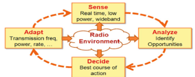
Fig. 4 Functional architecture of cognitive radio
