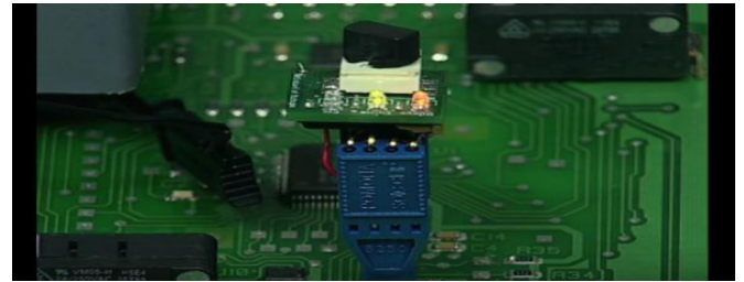
Figure 4. External device to rewrite the memory
