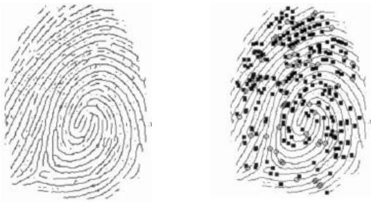
Figure 8 An original thinned fingerprint (left) and a copy of the image with all candidate minutiae represented on it (right). Squares represent ridge endings and circles represent bifurcations [21]
