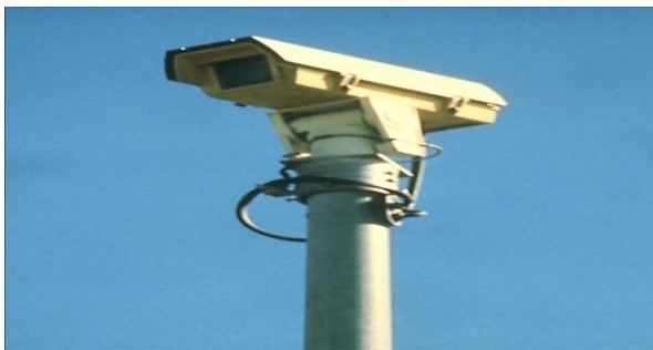
Pan, Tilt and Zoom (PTZ) Closed Circuit TV Camera (Image courtesy of the IBI Group)
