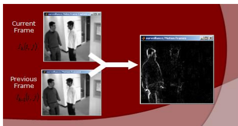
Fig. 2 Example of frame difference method
