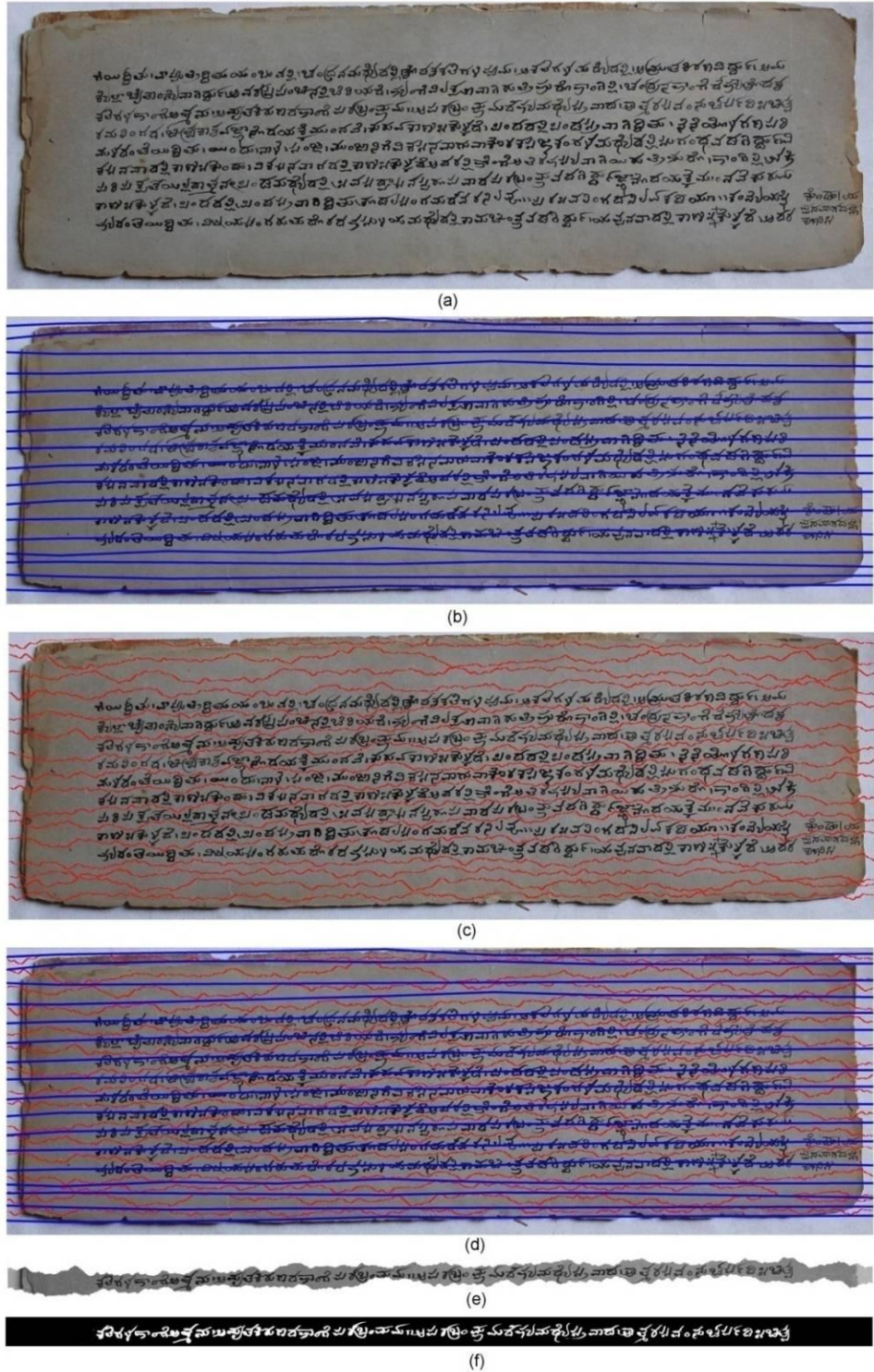
Figure 2. Sample image of the proposed algorithm (a) Original camera captured historical Kannada handwritten manuscript document image of Vijayanagara dynasty (1460AD) (b) medial seam computed image (c) Separating seam computation image with constrained seam carving based on medial seam (d) overlaid image with both type of seam (e) text line is extracted based on the overlaid seam (f) Enhanced and size normalized image
