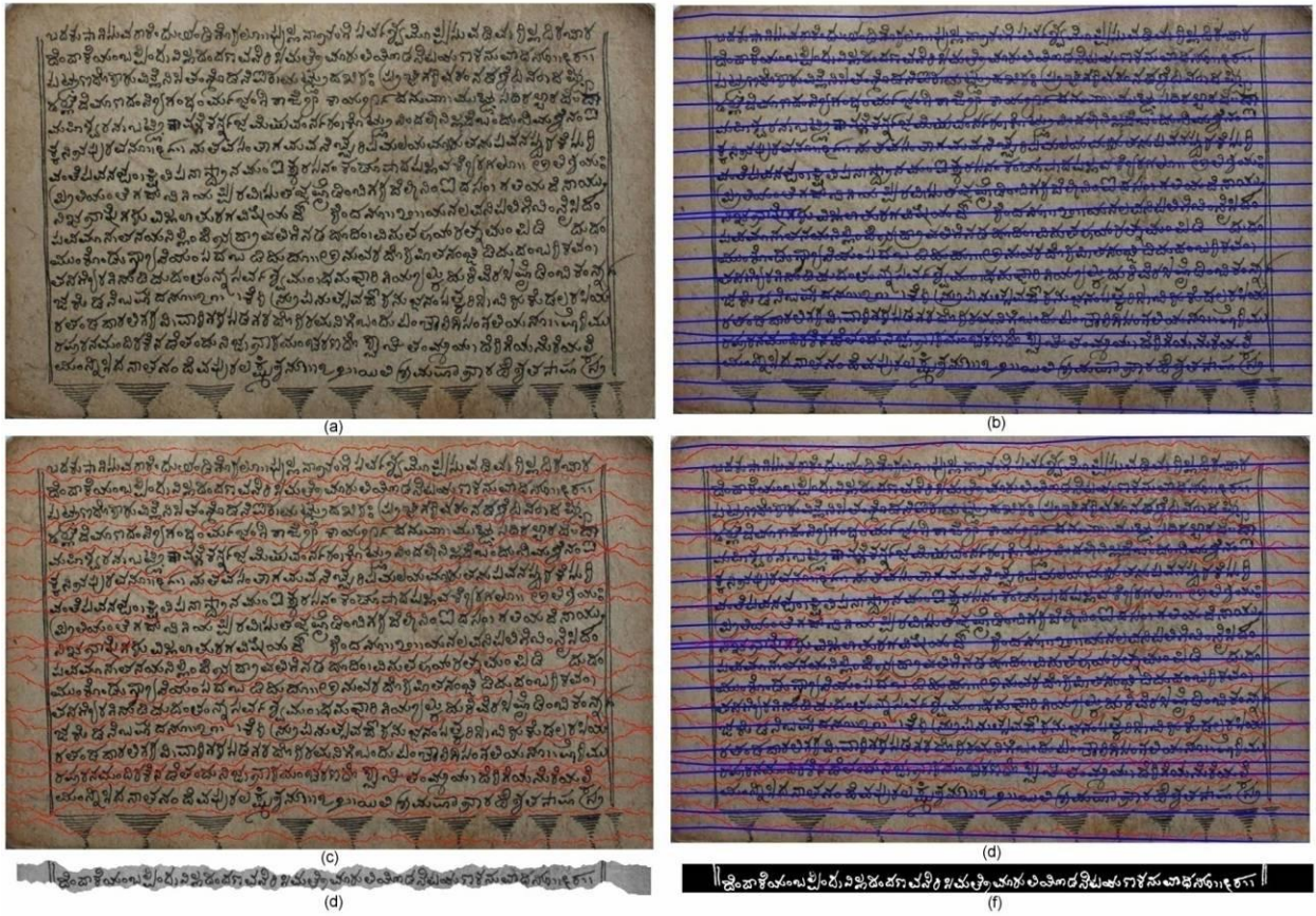
Figure5. Sample image of the proposed algorithm (a) Original camera captured historical Kannada handwritten manuscript document image of Hoysala dynasty (1340AD) (b) medial seam computed image (c) Separating seam computation image with constrained seam carving based on medial seam (d) overlaid image with both type of seam (e) text line is extracted based on the overlaid seam (f) Enhanced and size normalized image
