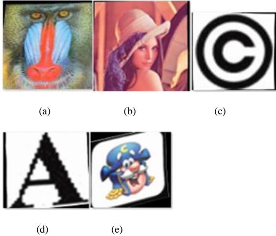
Figure 12 attack of after random distortion 0.95; (a) 2 nd watermarked image, (b) 1 st watermarked image, (c) retrieved watermark image 1 st , (d) retrieved watermark image 2 nd , (e) retrieved watermark image 3 rd .
