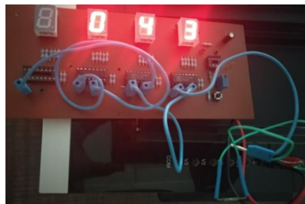
Figure.14. Tachometer design for Reed relay sensor
