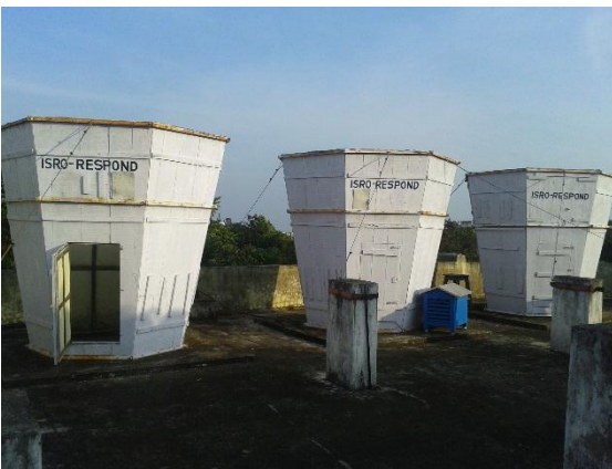
Figure.3: SODAR antenna at Dept. of Systems Design, Andhra University. Sponsored by UGC and ISRO.
