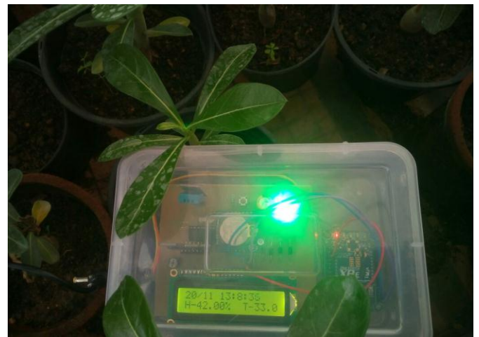
Figure 3 Sensor Node (Transmitter Module)
