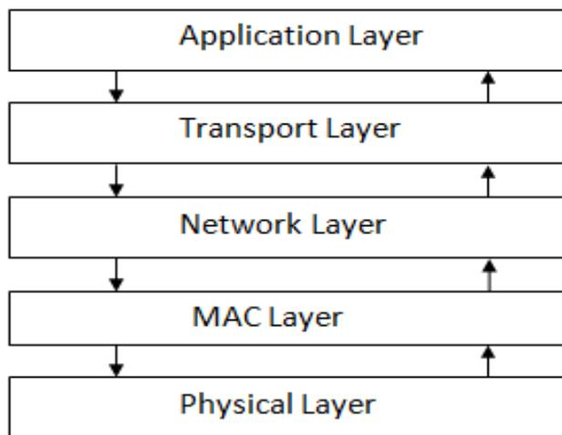
Figure 1. Wireless sensor networks protocol stack.
