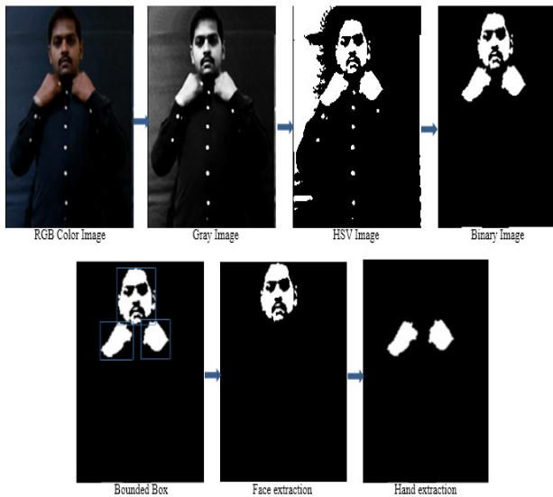
Figure 3. Shows pre-processing steps of each RGB frames from continuous gesture for the sentence “My father is in higher post”. (“ನನ್ನ ತಂದೆ ಹೆಚ್ಚಿನ ಪೋಸ್ಟ್ ಆಗಿದೆ”)
