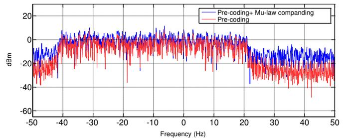
Fig.7 PSD of  $\mu$ -law companded Localized DFTS-OFDM which used zero padding in the end of bit stream (with  $\mu=255$ )
