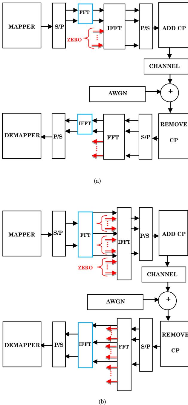
Fig.2 Block diagram of DFTS-OFDM system with (a) zero padding technique and, (b) zero interleaving technique
