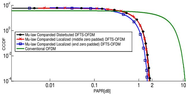
Fig.4 CCDF of various types of OFDM systems
