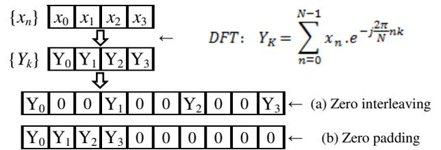
Fig.3 Example of zero insertion techniques in the frequency domain for  $N=4$  subcarriers with (a) zero interleaving, (b) zero padding
