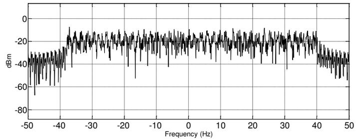
Fig.5 PSD of conventional OFDM system
