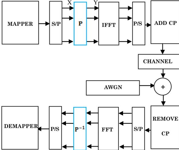
Fig.1 Block diagram of pre-coding based OFDM system
