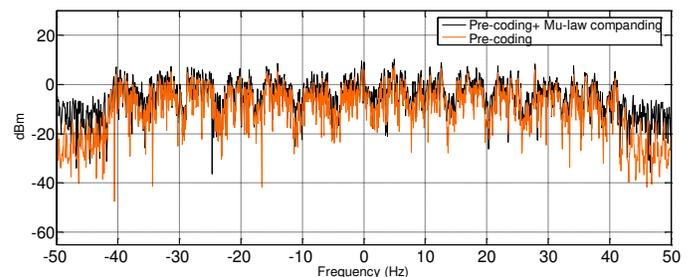
Fig.8 PSD of  $\mu$ -law companded Distributed DFTS-OFDM (with  $\mu=255$ )
