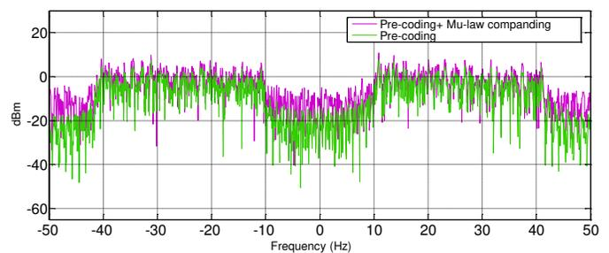
Fig.6 PSD of  $\mu$ -law companded Localized DFTS-OFDM which used zero padding in the middle bit stream (with  $\mu=255$ )
